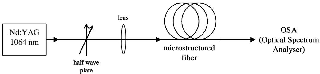
Fig. 1. Experimental set-up.
