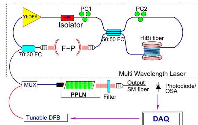
Fig. 2. Experimental setup. YbDFA, Ytterbium doped fiber amplifier; PC, polarization controller; FC, fiber coupler; F-P, Fabry Perot filter; HiBi fiber, high-birefringence fiber; DAQ, data acquisition system.
