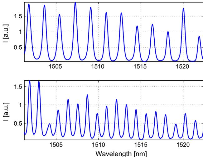
**Fig. 5.** Measured SFG power upon signal wavelength for various FSR of the MWL laser.
