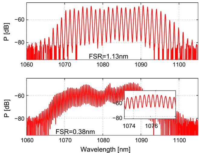
Fig. 3. MWL output spectrum for an FSR of 1.13 nm (top) and 0.38 nm (bottom). Inset: detail around 1075 nm.
