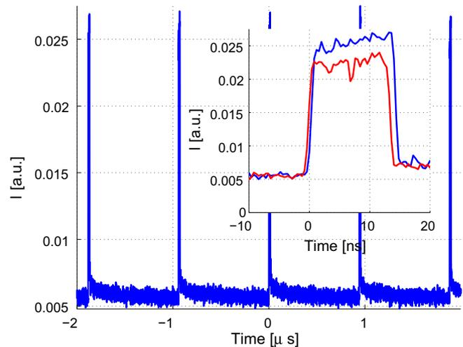
Fig. 4. Time domain analysis of the mode-locked regime. Inset: pulse duration with FSR = 1.13 nm (blue curve) and FSR = 0.38 nm (red curve). (For interpretation of the references to colour in this figure legend, the reader is referred to the web version of this article.)
