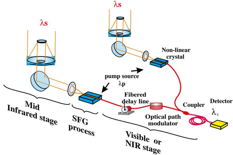
Fig. 1. General principle of ALOHA. The optical fields collected by a set of telescopes are frequency shifted in non-linear crystals into the visible or near infrared bands. The beams are then processed using optical fibers or guided components such as a fibered delay line and an optical path modulator. The two converted beams are mixed in a coupler and the fringe pattern is detected in the time domain by a silicon photon counting detector.
