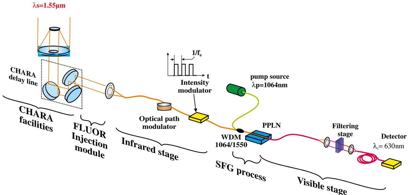
Fig. 3. Photometric configuration of only one arm of ALOHA at 1.55  $\mu\text{m}$  system implemented on the CHARA Array. An intensity modulator in the infrared stage is used to tag the star light signal.
