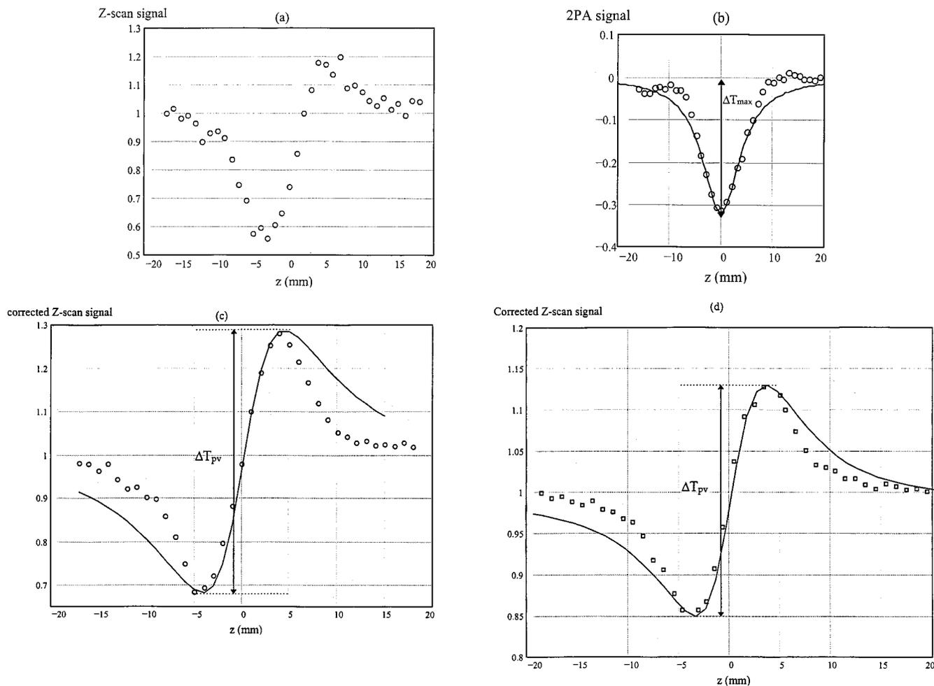
**Figure 3.** Normalized Z-scan curves: COPADR13:  $L = 2$  mm,  $D = 115$  mm,  $E = 233$   $\mu$ J. COPADO3:  $L = 1$  mm,  $D = 162$  mm,  $E = 182$   $\mu$ J.  $\circ$ , experimental data; solid curves, theoretical fitting. (a) COPADR13, uncorrected apertured Z-scan with  $S = 0.33$ ; (b) COPADR13, nonapertured Z-scan ( $S = 1$ ) featuring the 2PA; (c) COPADR13, corrected apertured Z-scan with  $S = 0.33$ ; (d) COPADO3, corrected apertured Z-scan with  $S = 0.03$ .
