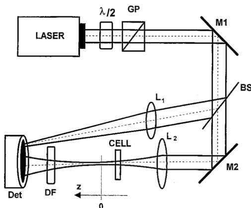
**Figure 1.** Schematic diagram of the experimental setup: pulsed Nd:YAG laser (LASER), mirrors ( $M_i$ ), half-wave plate ( $\lambda/2$ ), Glan polarizer (GP), beam splitter (BS), cell (CELL), converging lenses ( $L_j$ ), neutral-density filter (DF), CCD-camera (Det).
